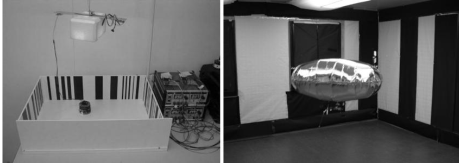
Fig. 1. Evolutionary vision-based robots. Left: The Khepera robot equipped with a linear camera (16 pixels, 36^\circ FOV) was positioned in an arena with randomly sized black and white stripes. Random size was used to prevent development of trivial solutions whereby the control system would use the size of the stripes to measure distance from walls and self-motion. The robot was connected to a workstation through rotating contacts that provided serial data transmission and power supply. Right: The blimp-like flying robot, provided with a similar linear camera (16 pixels, 150^\circ FOV), is closed in a 5 \times 5 \times 3 m room with randomly sized black and white stripes on the walls. The serial data transmission is handled by a Bluetooth wireless connection and power supply by an onboard battery lasting approximately three hours.
