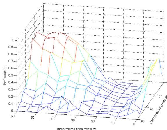
**Figure 5.19.** Varying the firing rates of correlated and uncorrelated synapses. Performance measured of three correlated synapses receiving SSIP input. In addition, twenty synapses receiving independent Poisson spike trains were added. Average over 10 runs.
