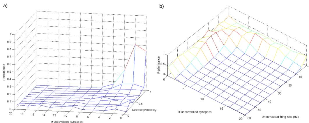
**Figure 5.18.** Effect of release probability and adding uncorrelated synapses receiving independent Poisson spike trains on performance. Performance measured of three correlated synapses receiving SSIP input at 20 Hz. Average over 10 runs. a) Varying release probability and number of uncorrelated synapses. Poisson rate of uncorrelated synapses is 20 Hz. b) Varying number of uncorrelated synapses and their firing rate. Release probability 1.0.
