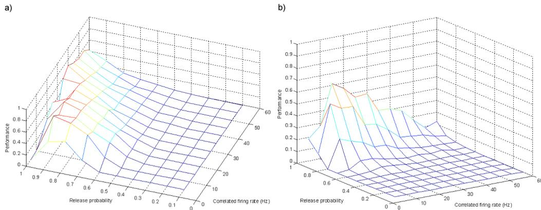
**Figure 5.29.** Varying synaptic release probability and input firing rate with 10 synapses. Performance measured of 10 correlated synapses receiving SSIP input. Average over 10 runs. a) No WSTDp, no dendritic decay. b) BPAP constrained WSTDp, dendritic decay.
