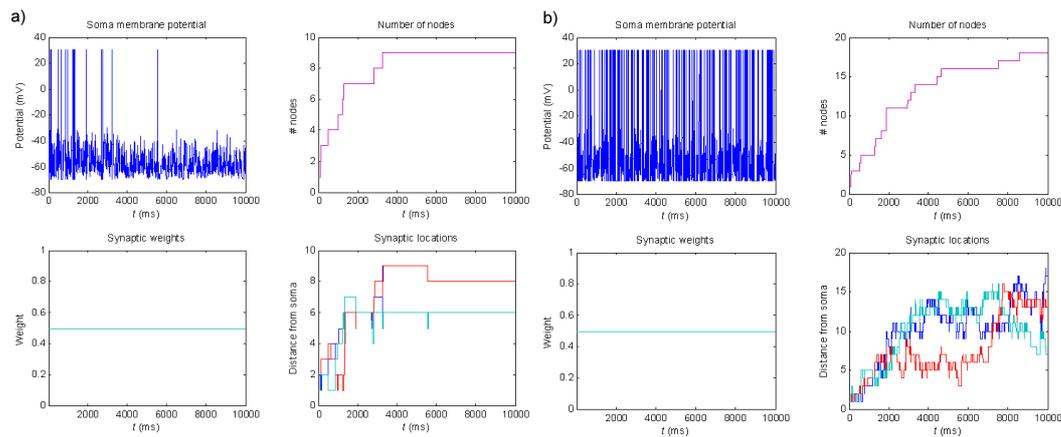
**Figure 5.9.** Two runs with three synapses receiving three Poisson inputs at 20 Hz, Box shaped LSTDp and no WSTDp. Top left: somatic membrane potential during the run; top right: dendrite length during the run; bottom left: synaptic weights during the run; bottom right: synaptic locations during the run. a) With dendritic decay. b) Without dendritic decay.
