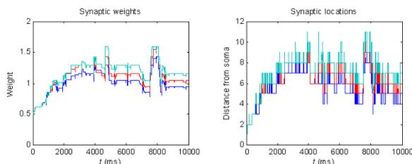
**Figure 5.14.** Synaptic weights and locations during a run with three synapses receiving SSIP input at 20 Hz, Box shaped LSTDP and BPAP constrained WSTDP. During large parts of the run, synapses are in the dispersed order (right). Furthermore, synaptic scaling is achieved: the weight of each of the synapses (left) is strongly correlated with synaptic locations (distance from the soma).
