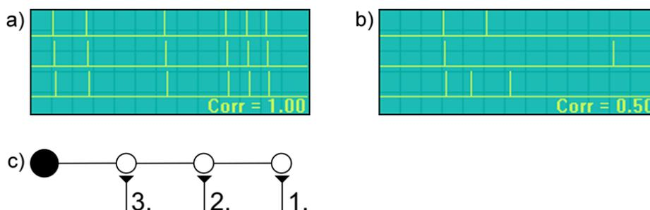
**Figure 5.20.** a) Three Skewed SIP generated spike trains with correlation 1.0. b) Three Skewed SIP generated spike trains with correlation 0.5. c) Synapses ordered on the linear dendrite based on the sequence in the input; compact order.
