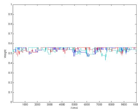
**Figure 5.10.** Run with three synapses receiving three Poisson inputs at 20 Hz, no LSTDp and BPAP constrained WSTDp. Synaptic weights are more or less kept between 0.5 and 0.6, keeping synaptic efficacies and thus output firing rate constant.
