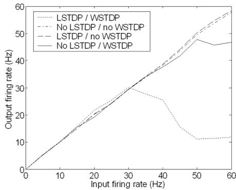
**Figure 5.15.** Effect of input firing rate on output firing rate with three synapses receiving SSIP input, Box shaped LSTDPA and BPAP constrained WSTDPA. The effect of four combinations of applying LSTDPA, WSTDPA and dendritic decay are shown. Average over 10 runs.
