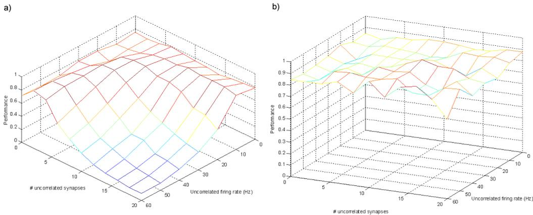
**Figure 5.25.** Varying the number of uncorrelated synapses and their firing rates. Performance measured of three correlated synapses receiving SSIP input at 20 Hz. Average over 10 runs. a) No WSTDP, no dendritic decay. b) BPAP constrained WSTDP, dendritic decay.
