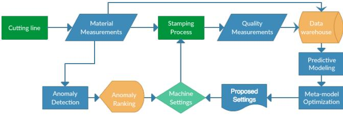
Fig. 1. A framework for optimizing and monitoring a car body parts manufacturing process.
